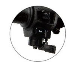
THANKS TO THE CHOKE MOUNTED WITHIN REACH ON THE HANDLE BAR, REGULATING THE AIR/FUEL MIXTURE IS CONVENIENT EVEN IN COLD WEATHER.
